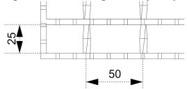
A grate's resistance against bicycle tyre penetration is often a primary concern in choosing grates for residential applications and so the EGAL range of trench and sump grates has been designed to exceed the BTPR requirements established in AS3996 - 2006.
