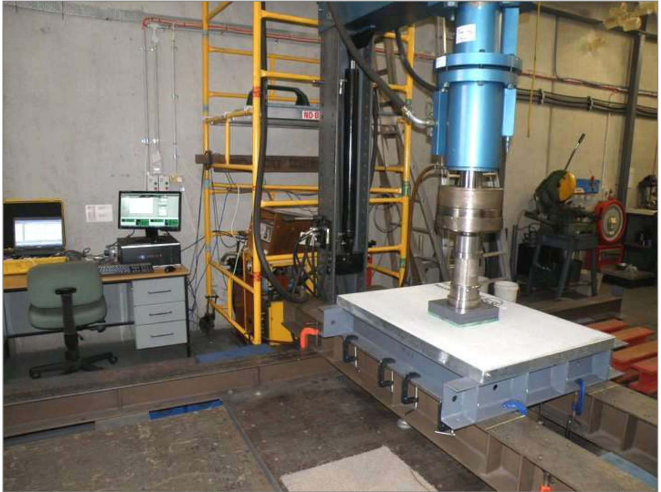
Fig. 2 COVER LOAD TEST SEP UP
